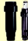
Toro 640 Series Sprinklers *Radius : 14-20M (47'-67') *Flow rate : 6.0-25.0 GPM 23-95LPM *Operating Pressure : 2,8-6,2 bar (40-90PSI)
